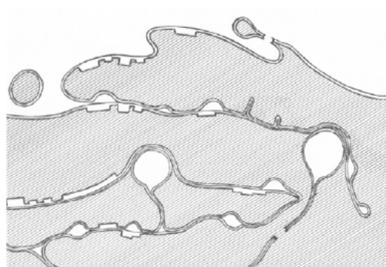
Different sizes of bi-films being created in a splash of metal, from a surface fold, and from impingement of droplets
