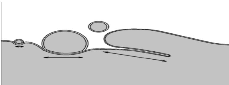
There are more than one steps in the production of metals in which the metal is consolidated from smaller fragments to make larger pieces for engineering purposes. In almost every case, the fragments have an oxide
